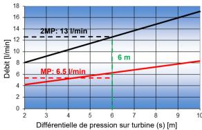
**Note:** The power supplied in the graph above is achieved by optimizing the power supplied by turbine(s) for each differential pressure. To limit the head loss, **the connection to the valve is recommended with size 3/8"(MP) and 1/2"(2MP)**.
