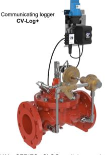
The CLA-VAL SERIES CLOG switches a latching solenoid by means of a CLA-VAL CV-Log+communicating logger, according to predefined rules, or upon remote command, via the CLA-VAL Link2Valves web platform.
