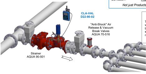
Recommended typical assembly for CLA-VAL automatic control valves
