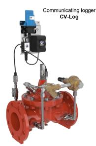
The CLA-VAL SERIES 90 COM reduces a higher inlet pressure to a constant downstream pressure (Pressure Reducing Control) regardless of changing flow rate and/or varying inlet pressure. It also integrates the CLA-VAL CV-Log communicating logger, allowing remote valve management and diagnostics, via the CLA-VAL Link2Valves web platform.
