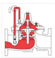
Tight Closing Operation: When pressure from the valve inlet is applied to the cover chamber, the
