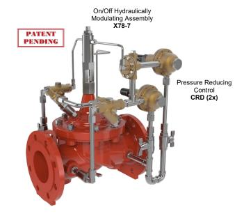
The CLA-VAL SERIES 98 Pressure Management Control Valve automatically adjusts the downstream pressure based upon demand changes in the system.
