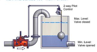
The CLA-VAL SERIES 100 On/Off Float Level Control Valve is a non-modulating valve which accurately controls the liquid level in a tank. This valve opens fully when the liquid level reaches a preset low level and closes drip tight when the liquid level reaches a high level.
