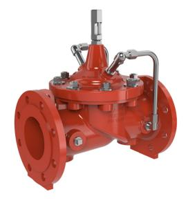
The CLA-VAL SERIES 81 is a hydraulically operated Check Valve. The valve opens when inlet pressure exceeds outlet pressure. In case of reversal pressure, the higher outlet pressure closes the valve to prevent backflow through the valve.
